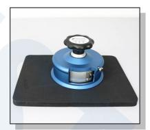
Circular sample cutter with cutting mat
