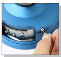
Pull it and rotate the side, cutter can be used.
